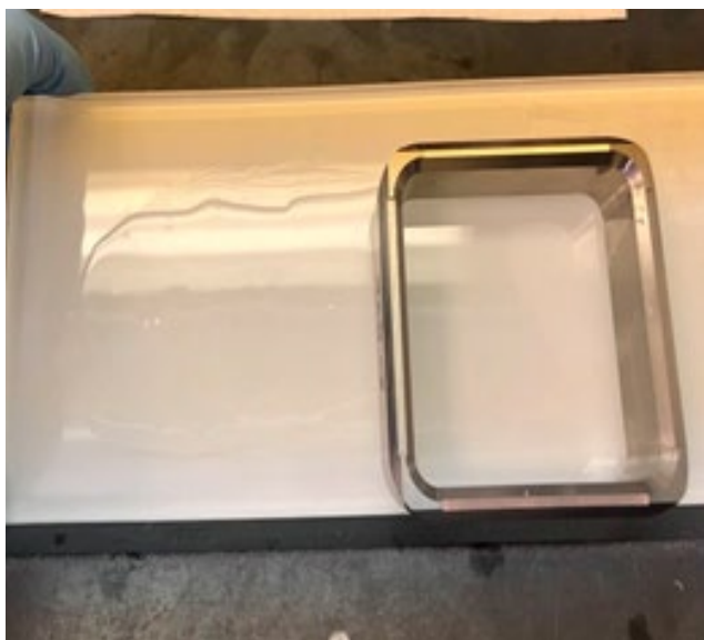
Figure 5.1 Multiple Clearance Square Applicator (Gardner, Pompano Beach, FL) used for polymer casting with eight different thickness controls (5mil, 10mil, 15mil, 20mil, 25mil, 30mil, 40mil, 50 mil).
