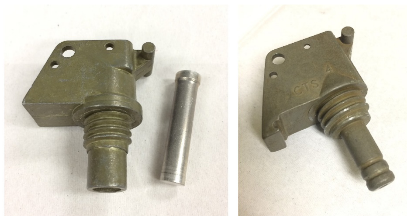
Figure ES-1. M201A1 (Left) and M213/M228 (Right) Fuze Configurations.
