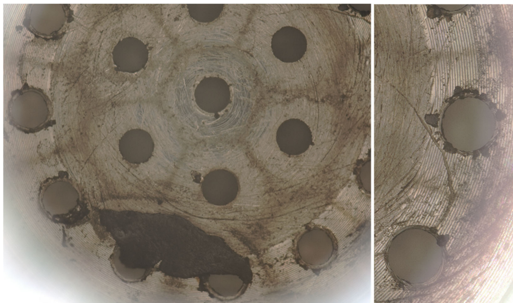
Figure 12. Photos of Orifice Plate at Conclusion of Testing With PFOS
