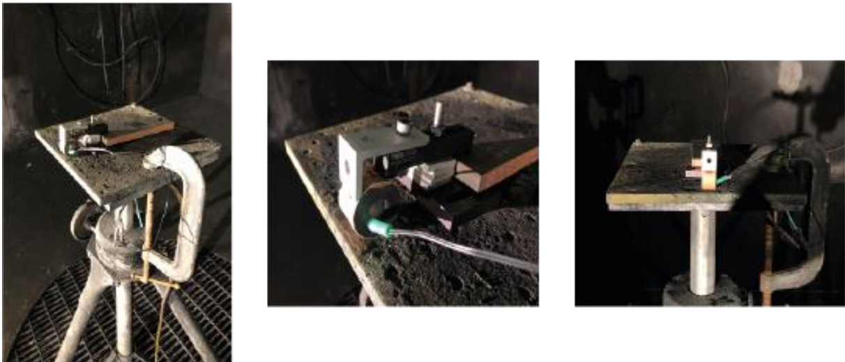
Figure 44: Set up for the measurement of the cluster flares; (left/middle) angled view, (right) frontal view.
