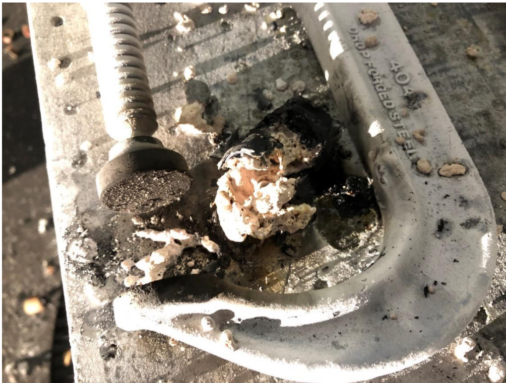
Figure 53: Composition I, which contained 33 wt-% \text{Li}_2\text{CO}_3 , produced large amounts of slag upon combustion, as shown by this photograph taken after a test of a parachute flare.
