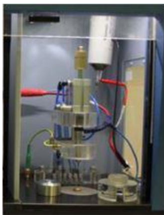
Figure 28: OZM Electric Spark Tester XSpark10 for measuring the electrostatic discharge.
