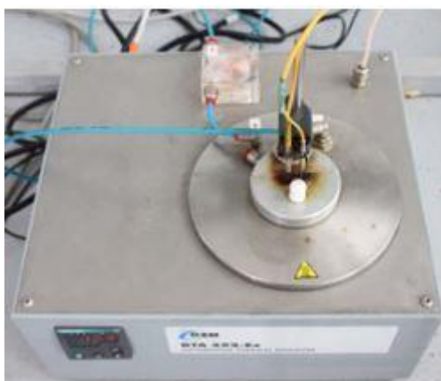
Figure 29: Differential thermal analysis device (DTA) for determination of decomposition temperatures.
