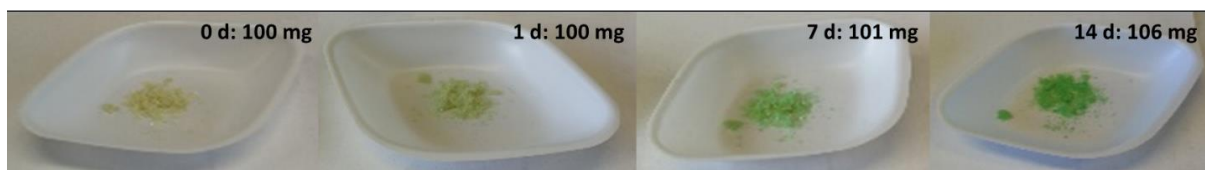
Figure 14: Change in color and weight of a sample of potassium dihydrobis(3-nitropyrzazol-1-yl)borate ( 51 ) after exposure to air for one, seven and 14 days, respectively.
