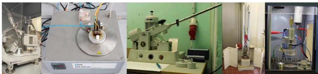
Figure 70: Analytical devices: Xcalibur Sapphire 3 for X-ray measurements, OZM DTA 552-Ex for differential thermal analysis, BAM standardized friction and impact device and an OZM Electric Spark Tester XSpark10, respectively.
