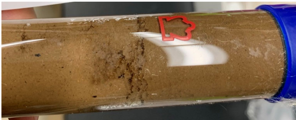
Figure 29. Soil A alkaline heat activated column effluent end.
