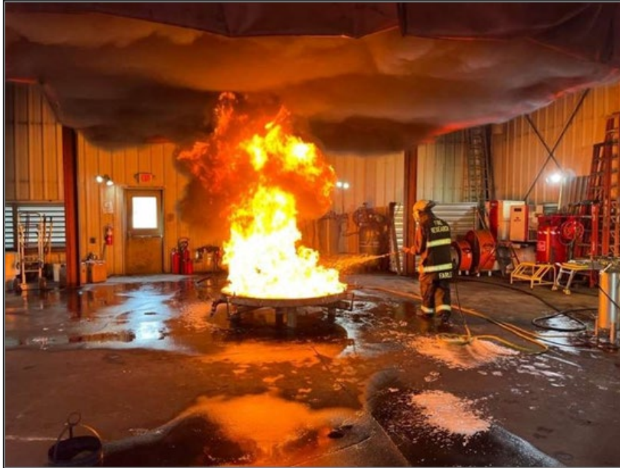
Figure ES-2. Ignited Fuel in 28 sq ft Pan and Application of Foam-additive Mixture
