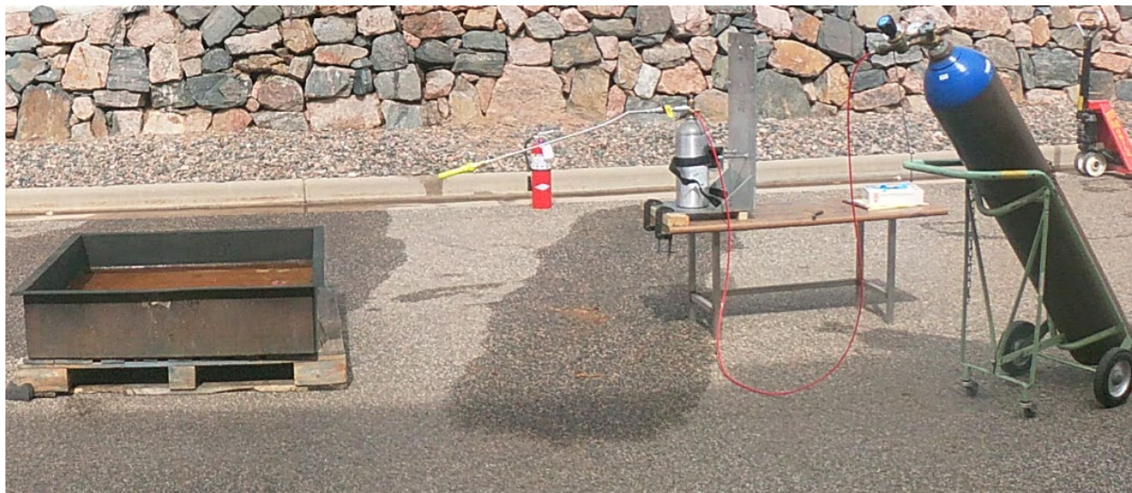
Figure ES-4. Setup of 12.5 ft² Fire Testing at ADA Facility
