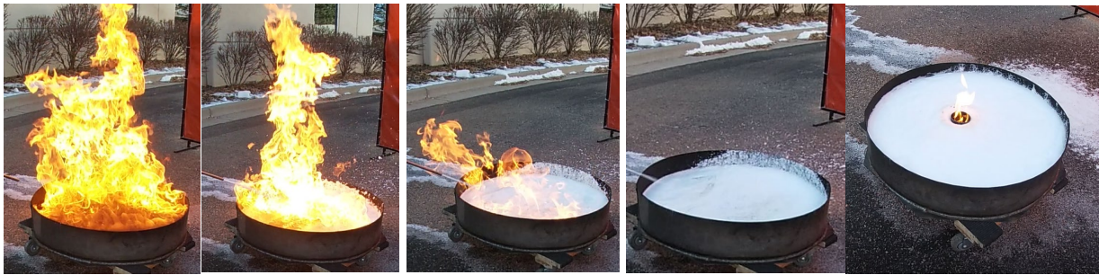
Figure ES-3. 5 ft² Class B Pool Fire (Heptane) Test with ADA Formulation
