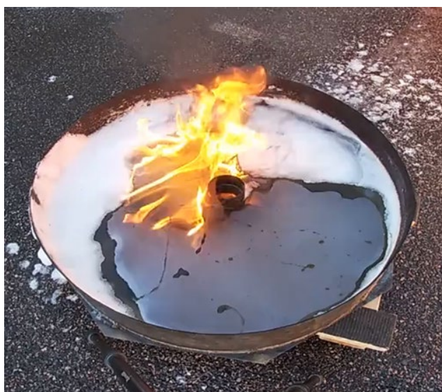
Figure ES-11. Film Formation Observed in Siloxane Ratio S1
