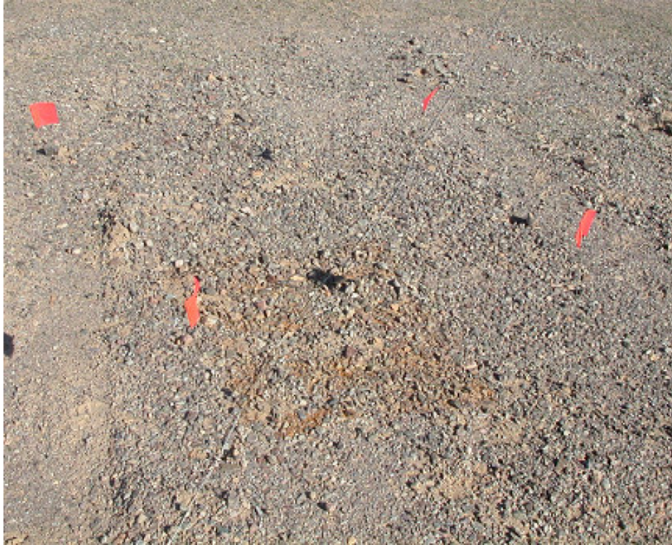
Figure 5. TNT-crystal contamination in Area 2.
