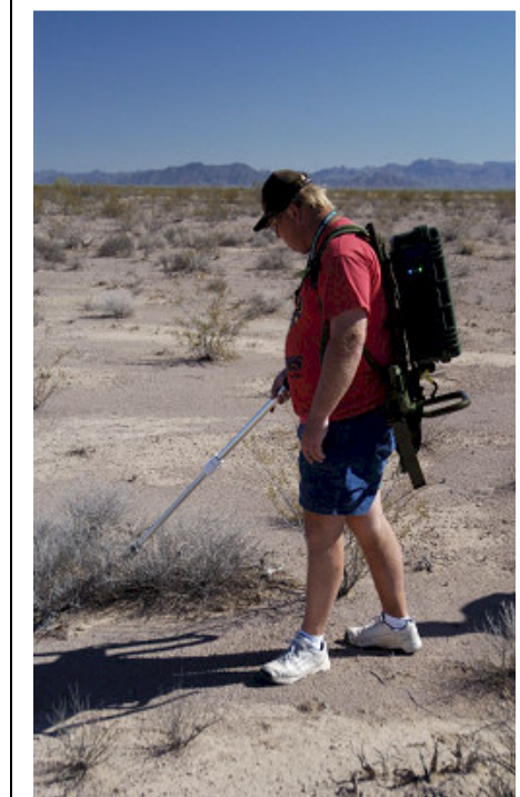
Figure 7. High-volume backpack sampler in use at YPG.
