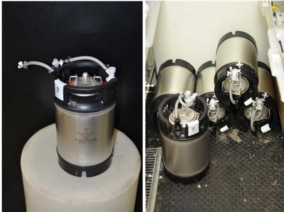
Figure 2.2.3-5. Mini-keg system being used to examine RDX degradation under selected electron acceptor conditions.
